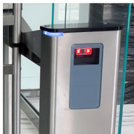
E. SIDE WINDOW Card reader mounted behind frosted acrylic window.
