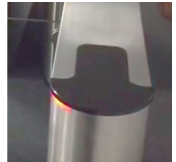
Figure 2: Flashing light indicates alarm has been triggered
