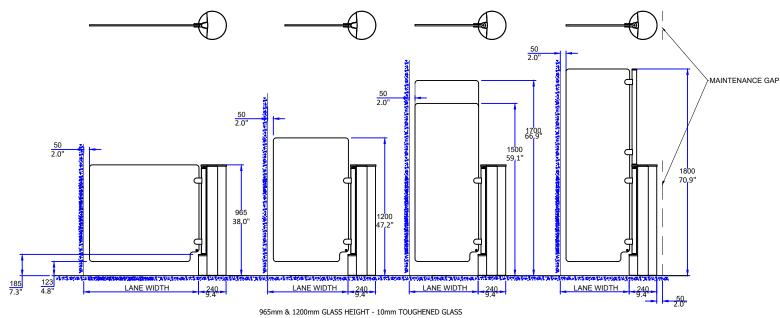
$1500 \mathrm{mm}$  &  $1800 \mathrm{mm}$  GLASS HEIGHT - TWO PIECES OF 5 mm TOUGHENED GLASS WITH 1.5 mm LAMINATE FILM IN BETWEEN
