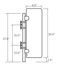
The Fastlane Wall Mounted Infill is available for gaps minimum of  $11.8^{\prime\prime}$  (300mm) to a maximum of 20" (500mm). Available in 1000, 1500, and 1800 tall Infill.
