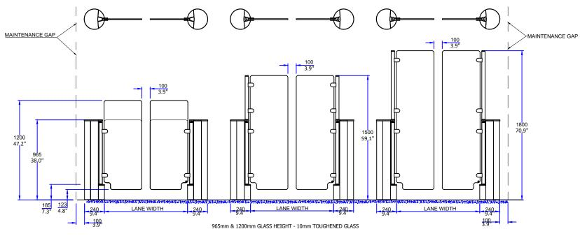
1500mm & 1800mm GLASS HEIGHT - TWO PIECES OF 5mm TOUGHENED GLASS WITH 1.5mm LAMINATE FILM IN BETWEEN
